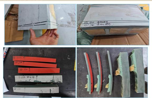
Combining the above characteristics, and comprehensively considering environmental protection, labor, safety, cost, efficiency and other aspects, the ultra-high pressure waterjet intelligent cutting solution is very suitable for the cutting needs of fiberglass workpieces in the wind power industry.
