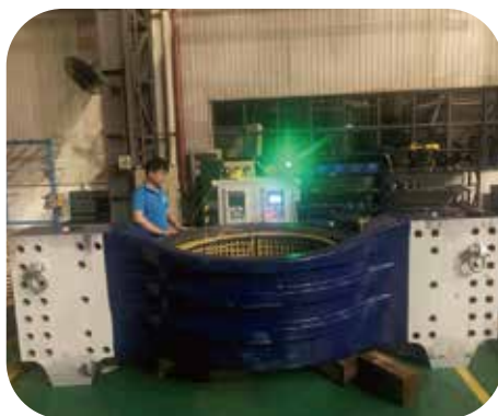
Heating bearing housing for mounting
