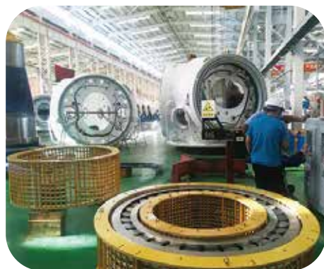
Heating bearing inner&outer ring for mounting
