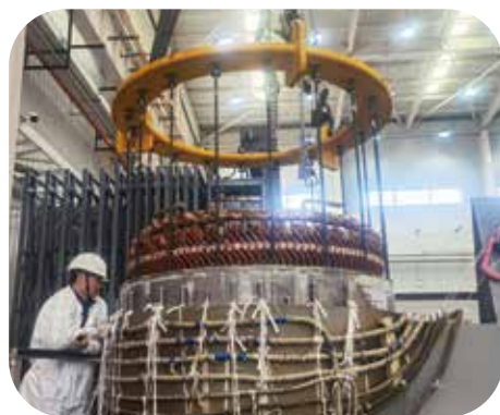
Heating motor housing for dismounting
