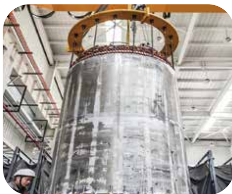
Heating motor housing for dismounting
