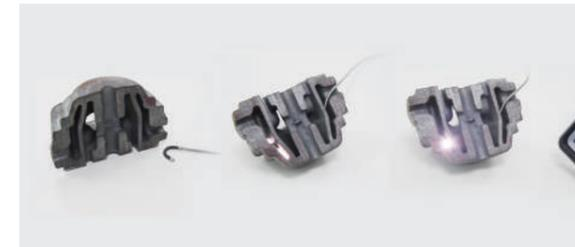
The special flexible insertion tube is equipped with a very thin probe, which can pass through the winding complex cavity.
