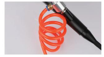
Equipped with cooling device, the probe can enter the high-temperature area for observation.
