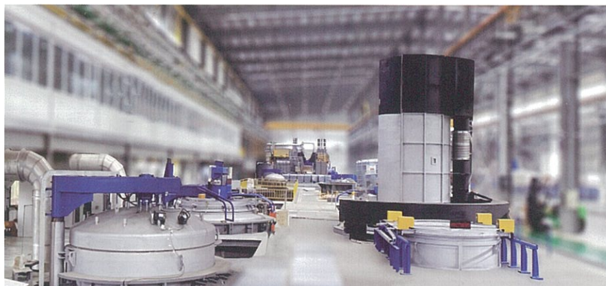
▲ 可控气氛井式渗碳炉热处理生产线 Atmosphere Pit Carburizing Furnace Line
