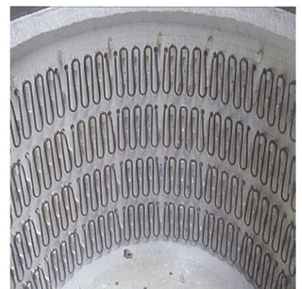
▲ (爱协林自主研发技术) 具有自脱碳功能的管状加热系统 Tubular Heating System with Self Decarburizing Function
