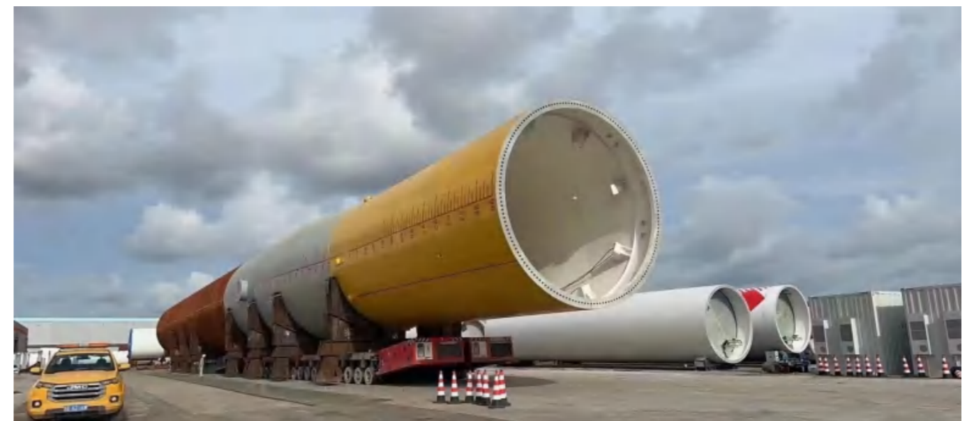
Monopile for 9MW Turbine SHENERGY C22 Offshore Wind Power Demonstration Project
