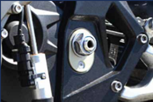
Full floating axle rear swinging
