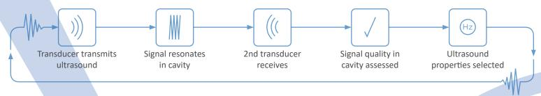
The sensor inherently compensates for changes in the air's temperature, pressure or humidity. A strong resonating sound wave in a small space provides a large signal that is easy to measure. Acu-Res® has a signal to noise ratio more than 40dB stronger than other ultrasonic technologies.
