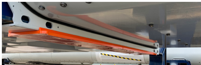
Polyurethane pad with embedded magnets to protect nacelles during transportation.
