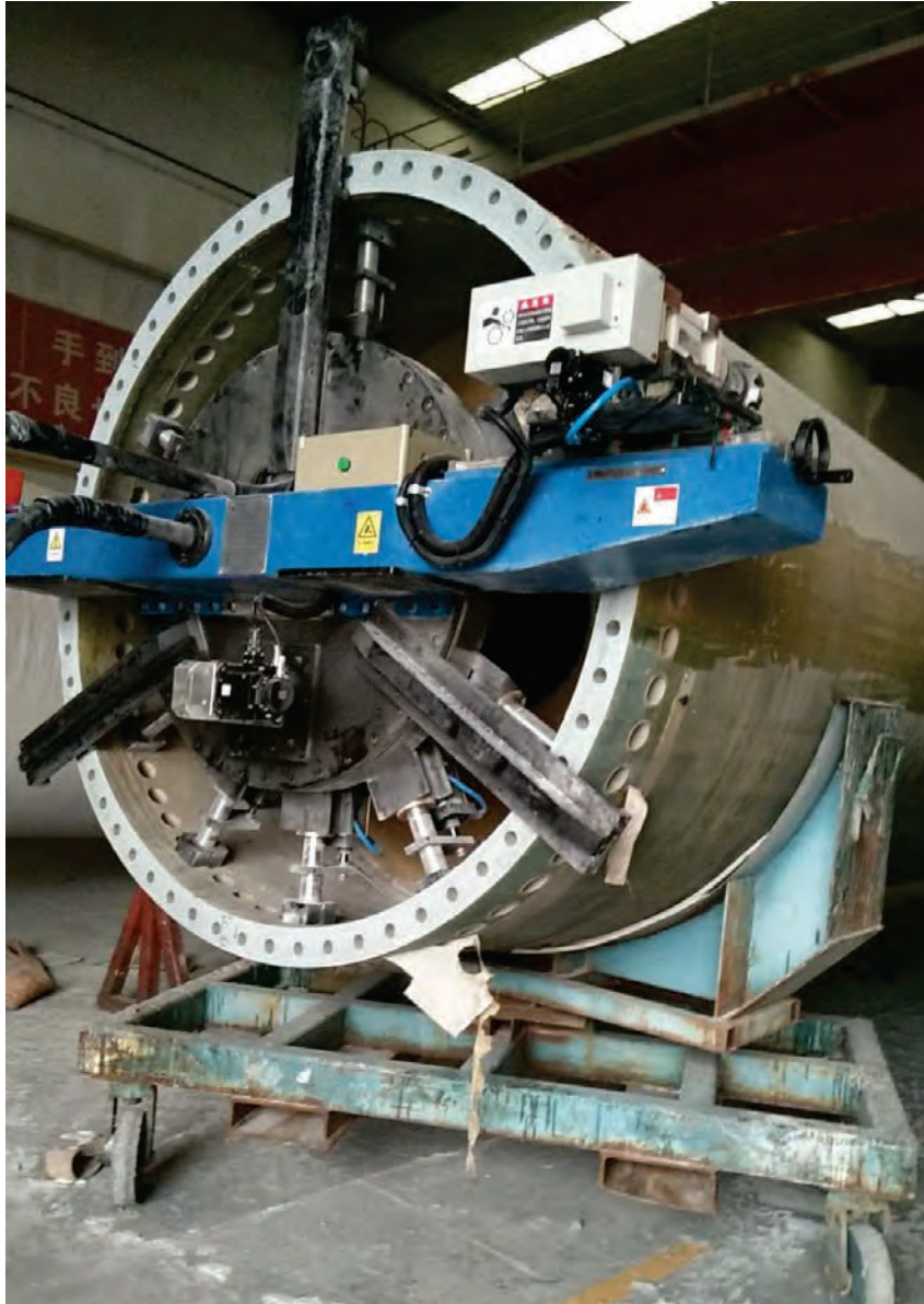
Fig. 11 end face milling machine process (drilling blade root)
