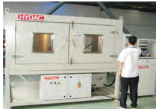
Oil Pressure Pulse test 油脉冲试验
