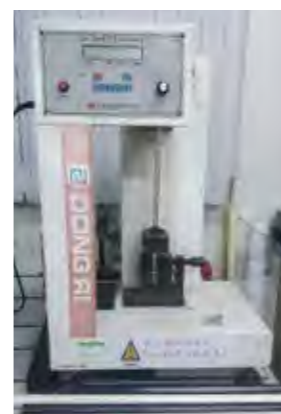
↑ 悬壁冲击实验机 Suspension wall impact test machine
