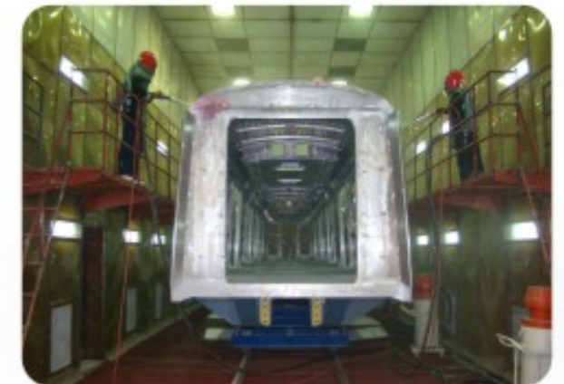
Railway Locomotive shotblasting Booth
