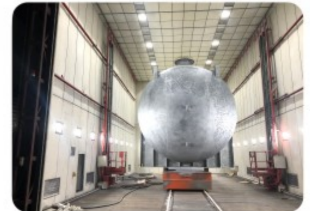
Chemical Container shotblasting Booth
