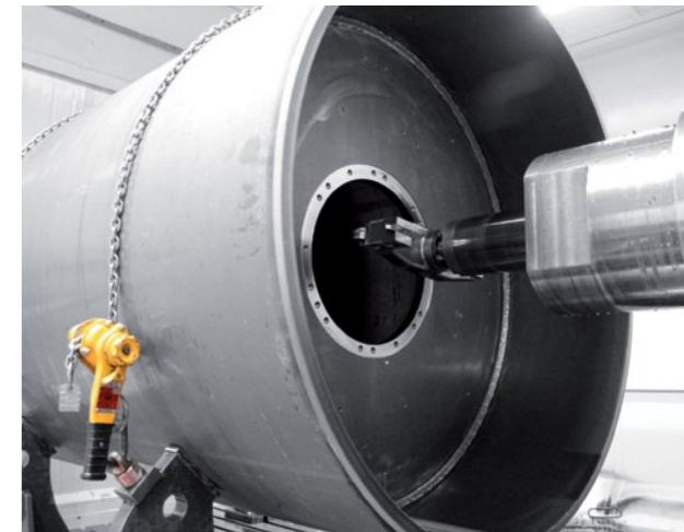
Fine machining of bore axis to fit H7.
